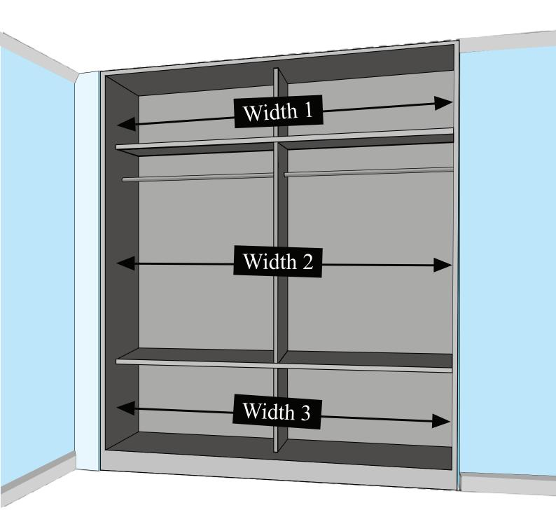
• Measure widths of the wardrobe at three different points as Top(Width 1), Middle(Width 2), and Bottom(width 3) as shown in the above diagram and the dimensions should be taken in Milli Metres (mm).
