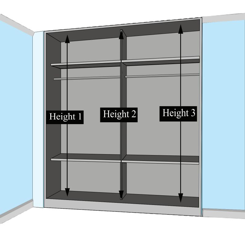
• Measure heights of the wardrobe at three different points as left(Height 1), Middle(Height 2), and Right(Height 3) as shown in the above diagram and the dimensions should be taken in Milli Metres (mm).
