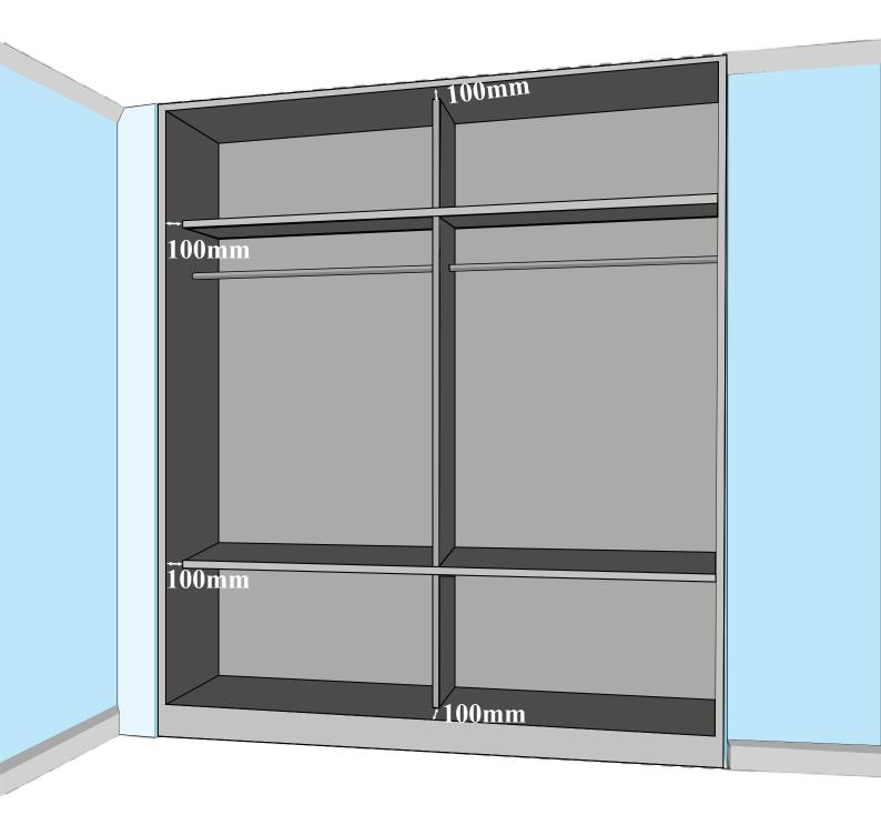
• To fit the sliding doors, 4inches(100mm) cleareance space should be left on all sides of the wardrobe as shown in vthe above diagram.
